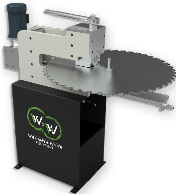
*The Williams & White Dish-O-Matic Stretcher Roll is essential in all saw production and maintenance facilities. The patented Dish-O-Matic system allows operator to tension and level saws in the most efficient and accurate manner. This machine is the most durable in the industry and is installed in thousands of filing rooms and saw shops worldwide.*
